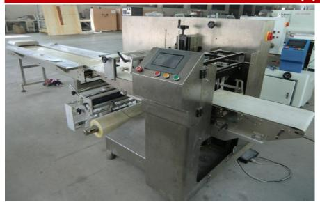
The BPS-700-WXSE is the perfect flow wrapper for wide products like <u>Tortillas, Flatbreads, Pizzas</u> and more. A bottom film wrapper, the BPS-700-WXSE can wrap stacks and irregularly shaped product.
